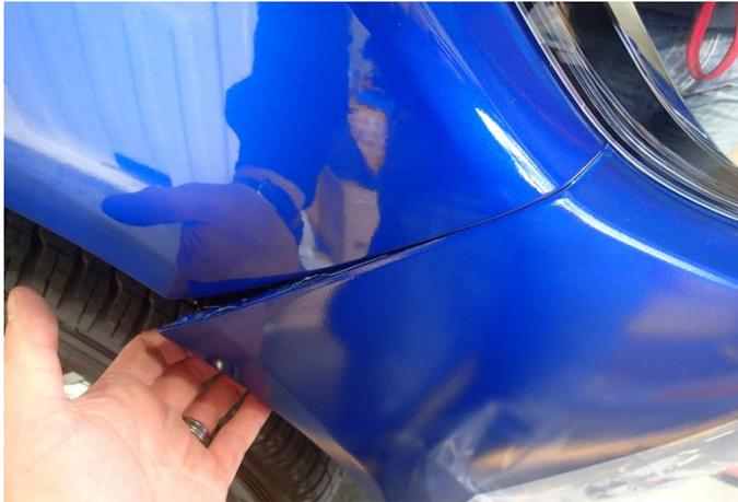
11. Remove registration plate and set aside, then carefully remove bumper from vehicle by pulling on each side of the bumper near the wheel arches and working your way towards the centre.
