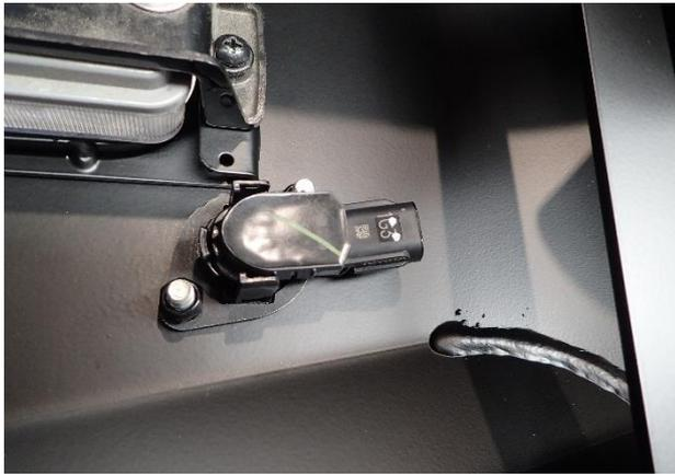
66. Fasten assembly to bullbar by torquing M6 Nyloc nuts to specification. Remove dome plugs and press RHS sensor into black retainer. **CHECK SENSOR IS CONCENTRIC IN HOLE, IF NOT ADJUST.**
