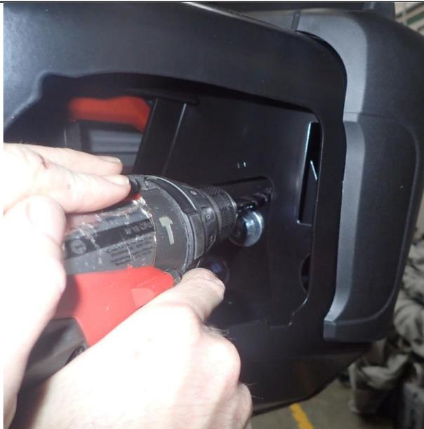
74. Drill 4 x Ø10mm holes (2 per side) through mount assembly using existing holes in bull bar as guide.
