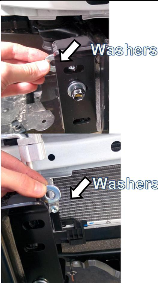
39. On both RH and LH installation it is extremely important that 1 x M10 x 25 x 3mm flat washer per hole is installed on the upper holes between the support brackets and the mount when offering the mount up to the chassis flange. The upper M10 bolts as installed in step below should pass through the mount, spacer washers and the support brackets.
