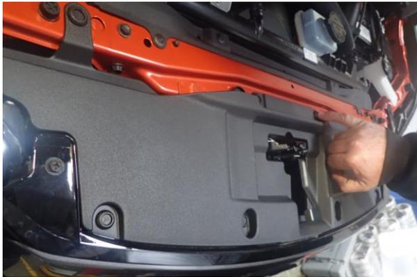
89. Re-install upper radiator cover panel and fasten using 8 x OE scrivenets.
