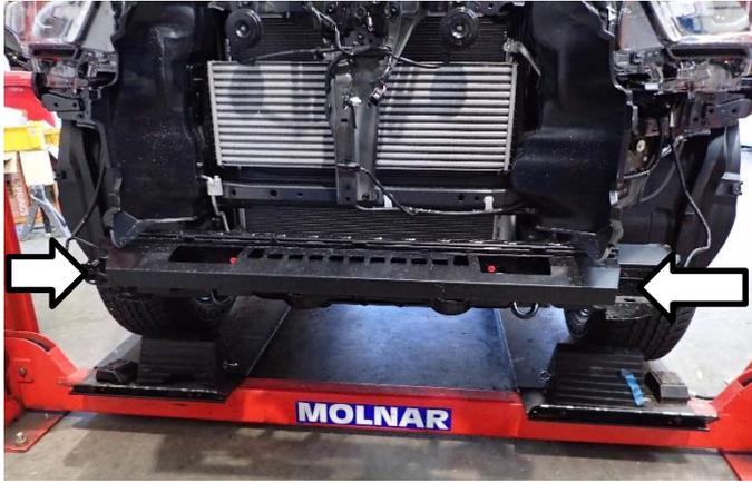
14. Remove plastic lower impact absorber from vehicle and discard.
