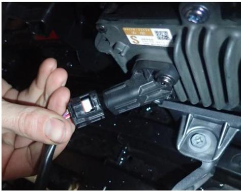
32. If vehicle is equipped with adaptive cruise control, reconnect radar.
