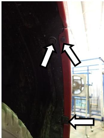
5. Remove all fasteners and scrivets retaining bumper along inside edge of wheel arches – (Right hand side shown).
