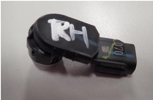
12. Using a paint pen or white marker, label each parking sensor (Left or Right) prior to removing from bumper.
