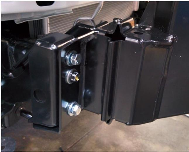
70. Adjust position of bar left/right until it's sitting central to body, then tighten all fasteners joining mount assembly to chassis brackets (4x M10 and 2x M10 OE bolts each side).
