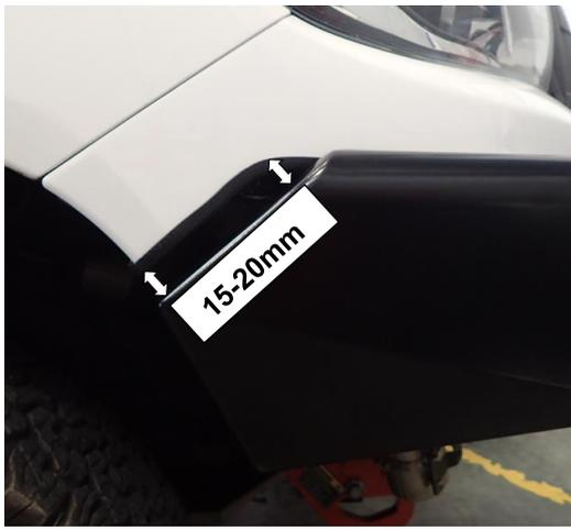
72. Position the bar so that it is level with the bumper cut profile as shown and there is an even gap of 15-20mm between the wing edge and bumper cut trim.
