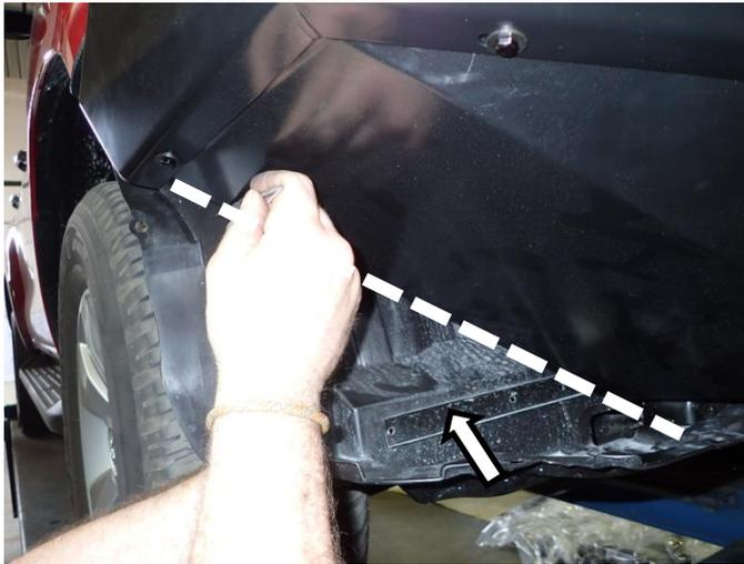
85. Mark lines onto the OEM inner guards (LH & RH) using lower edge of wing under panels as guide ensuring enough guard remains so that it may be neatly tucked/secured behind wing under panel lip.
