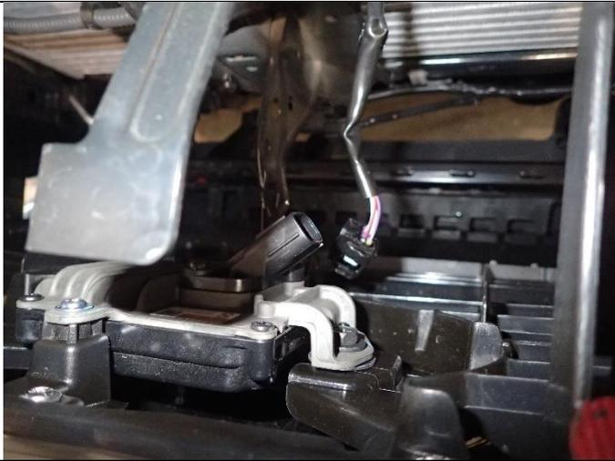
8. If vehicle is equipped with adaptive cruise control, unplug radar (located behind Toyota badge)
