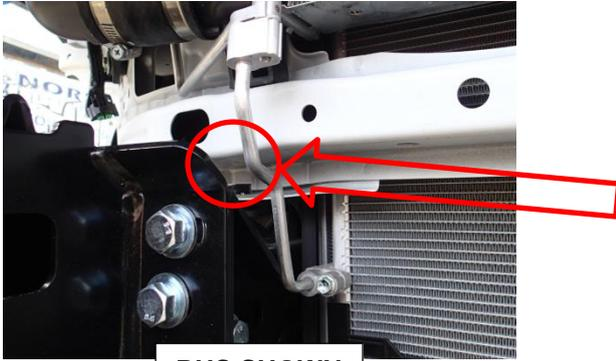
43. Loosely install 2 x M12 x 35 bolts and flat washers through lower mount and chassis support brackets into M12 flange nuts.
