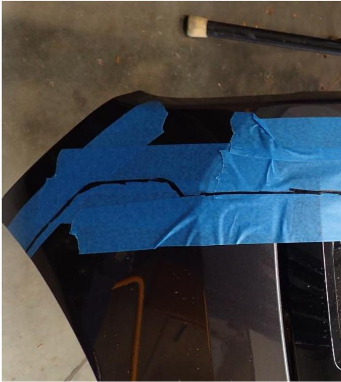
22. Stick masking tape onto bumper at area underneath headlight as shown running the tape well in towards the centre of the bumper.
