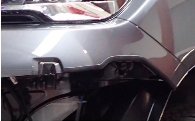
33. Fit Pinch weld to RH side along the full length of the cut edge. Carefully trim off any excess length and use remainder for other side.
